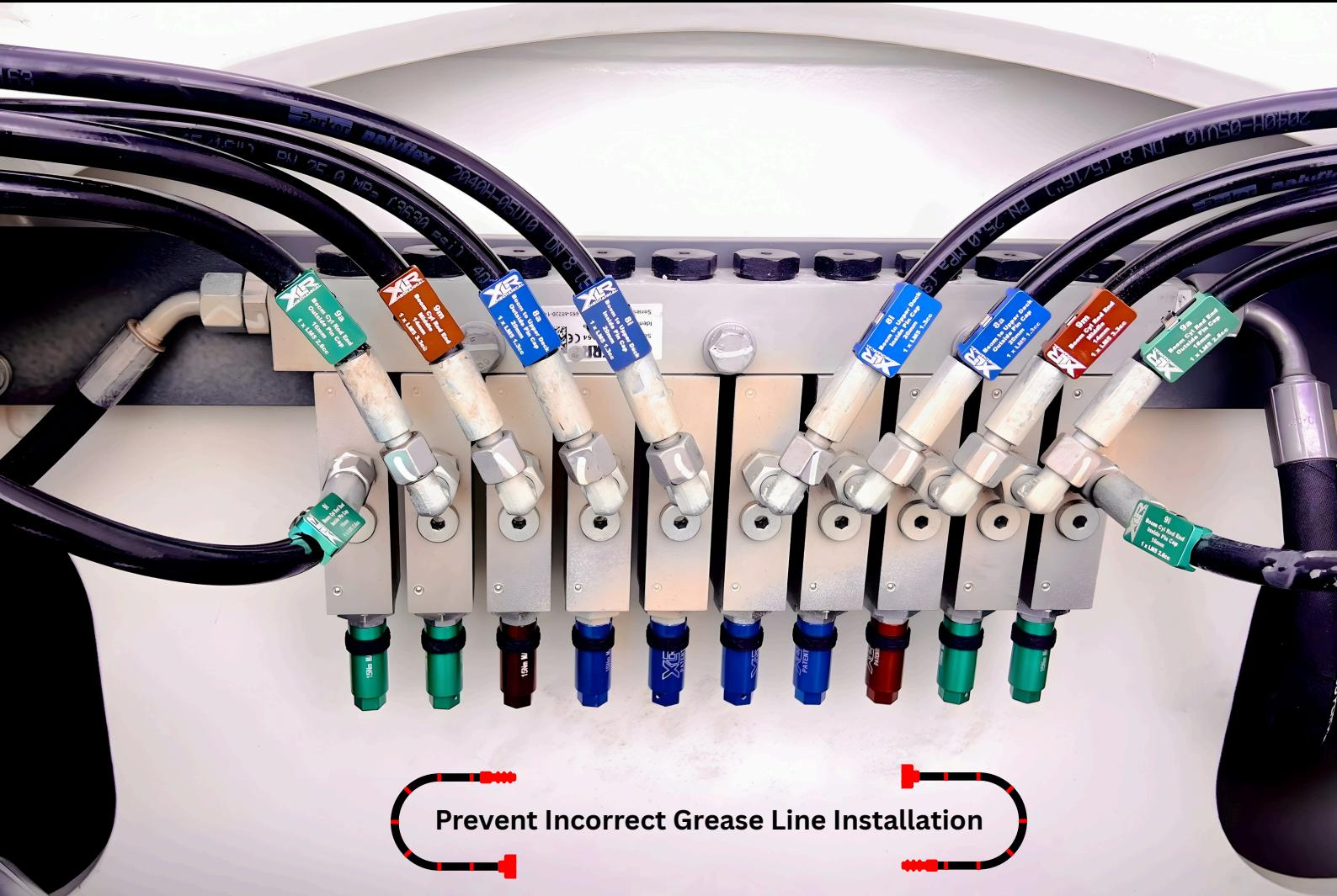
Prevent Incorrect Grease Line Installation
